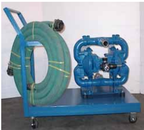
MART EQ-1 Transfer Pump & Cart Assembly. Two (2) inch diameter Flap Valve Air Operated Diaphragm Pump mounted on cart with swivel casters and brakes. Has 15 ft Inlet Hose and 15 ft Outlet Hose with 1.5" male and female Quick Disconnects to mate with the MART EQ-1 Processor. Pump has adjustable flow rate up to 140 GPM.
