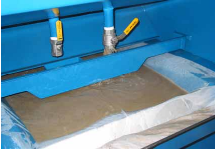
Draining encapsulated waste onto the filter paper
