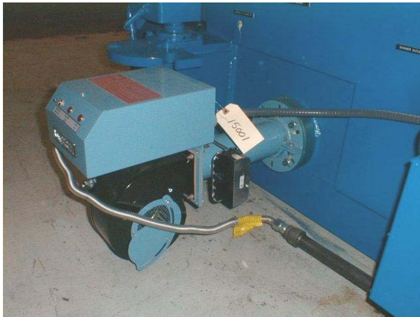
Fig. 5 - 7: Burner Blower Motor (380,000 BTU Burner Shown; Other Sizes Similar)
